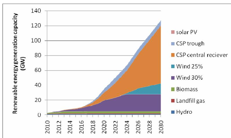
Figure 15: Renewable energy generation capacity development to 2030 under Roadmap 3
