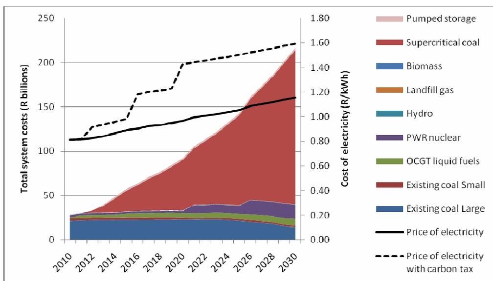
**Figure 6: Total system cost and average cost of electricity for the baseline scenario**
